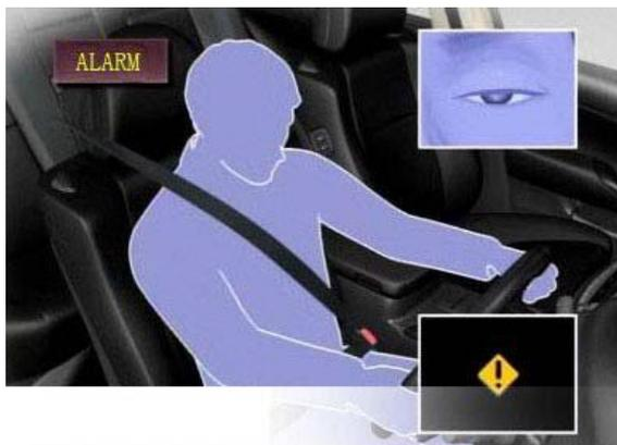
The EA-430 driver fatigue alarm system is the most advanced non-contact method to capture infrared images of people's eyes and the PERCLOS algorithms alerts the driver in time to protect your life and property.
